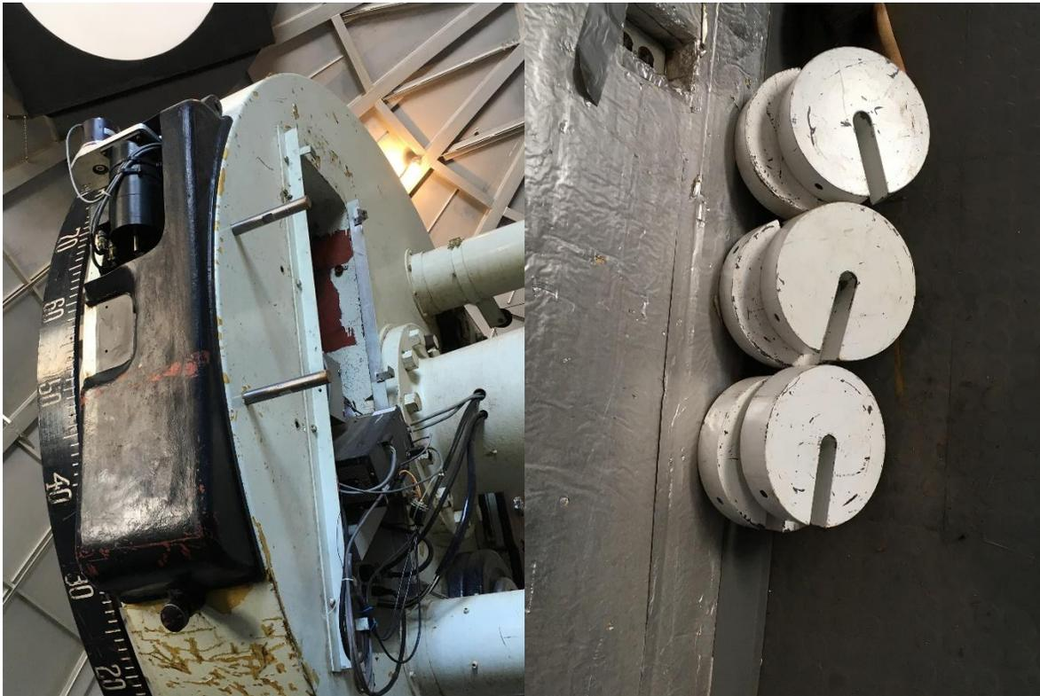
Two arc shaped weights were tied to one end of the ballast. The tape value is then 45-3/4”:
