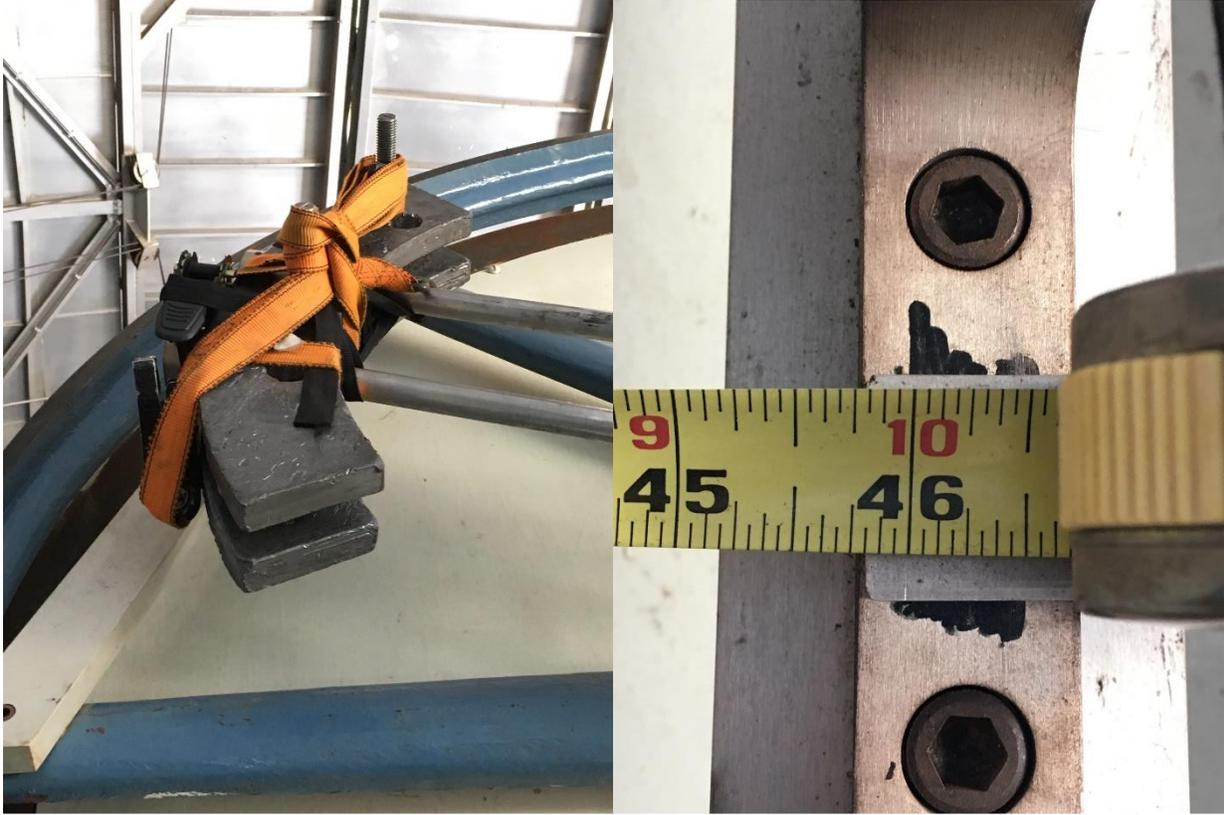
Two white balance weights C and D are set at zero, all the way to the end of their reach. A and B balance weights are set at 18.
